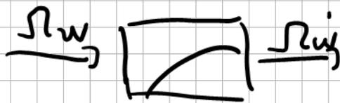
$$F_{WF} = \frac{1}{1 + T_{zn} \cdot s} = \frac{1}{1 + a^2 T_{on} \cdot s}$$
