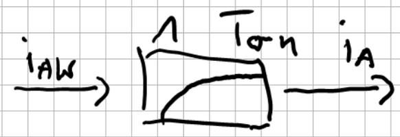
$$F_{on}(s) = \frac{1}{1 + \frac{2d}{\omega_0} s + \frac{1}{\omega_0^2} s^2} = \frac{1}{1 + 2t_T s + 2t_T^2 s^2}$$
